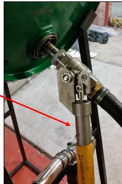
Competitors must ensure this refuelling rig arrangement is properly secured to ensure it cannot be fall, or be dragged over, in the Event of an incident. This rig is not to be moved after it has been filled. No part of the storage container, except for any venting system shall be at a height above 2.00m from the garage/pit bay floor.
